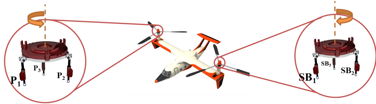
Swashplate actuator movement
